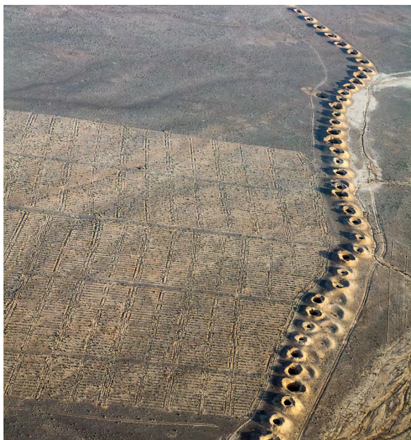
A line of evenly spaced spoil craters snake along the surface of the desert from the high Elburz Mountains to the Plains of Iraq and is the only evidence of an invisible, subterranean man-made water stream called a qanat , first constructed by the Persians during the early years of the first millennium BCE.
