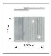
Z-Clips can be used for conditions where GATHER Acoustical panels will need to be removable from walls. Z-Clips are 1-1/2" wide and approx. 2" high. Z-Clip Rails are 72" long. Both are available from Wolf-Gordon.
